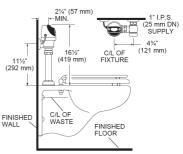
When installing the Sloan ECOS® Hardwire in a handicap stall:
